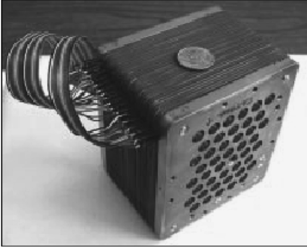
FIGURE 16.22 Direct methanol fuel cell stack (30 units). (Department of Energy, “Direct Methanol Fuel Cell,” http://www.ott.doe.gov .)
